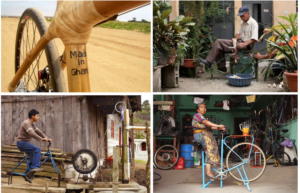
Illustration P.6 (from top left to bottom right): a bamboo bicycle ( https://www.ghanabamboobikes.org ); a bicycle mill; a bicycle rope water pump; a bicycle blender ( https://www.bicimaquinas.com ).
