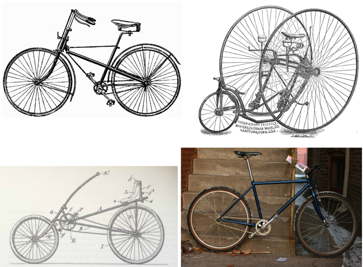
Illustration 4.4: 'Rover' safety bicycle from 1886 (reproduced from Lexikon der gesamten Technik 1901); The Coventry Rotary tricycle from around 1884 (reproduced from Tricyclists indispensable annual and handbook 1883); patent for a recumbent bicycle from 1895 (reproduced from Hadland and Lessing 2015);
